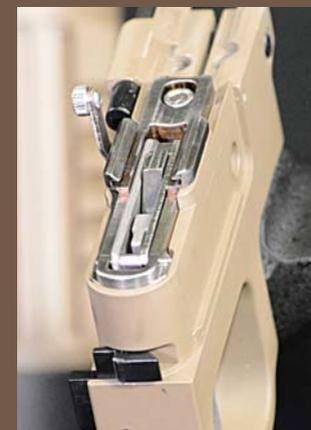
control group can be removed in simple rearward motion with the removal of a single screw from the receiver. Features ambidextrous magazine release.
