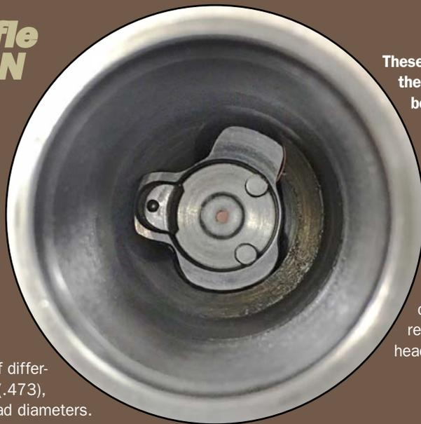
These rear-centering features combine with the aforementioned bolt lugs to allow the bolt to remain static when fired.
